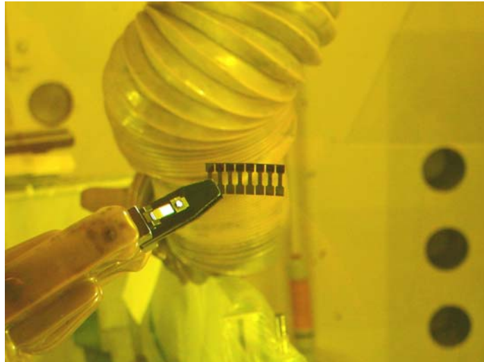
Figure 2.7. Electro-erosion cutting of tensile test specimens of the in-service material inside a hot cell using manipulators.
