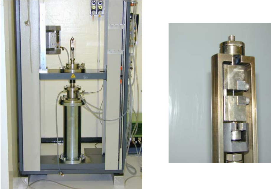
Figure 2.9. The ZWICK Z010 tensile testing machine and the specimen grips.
