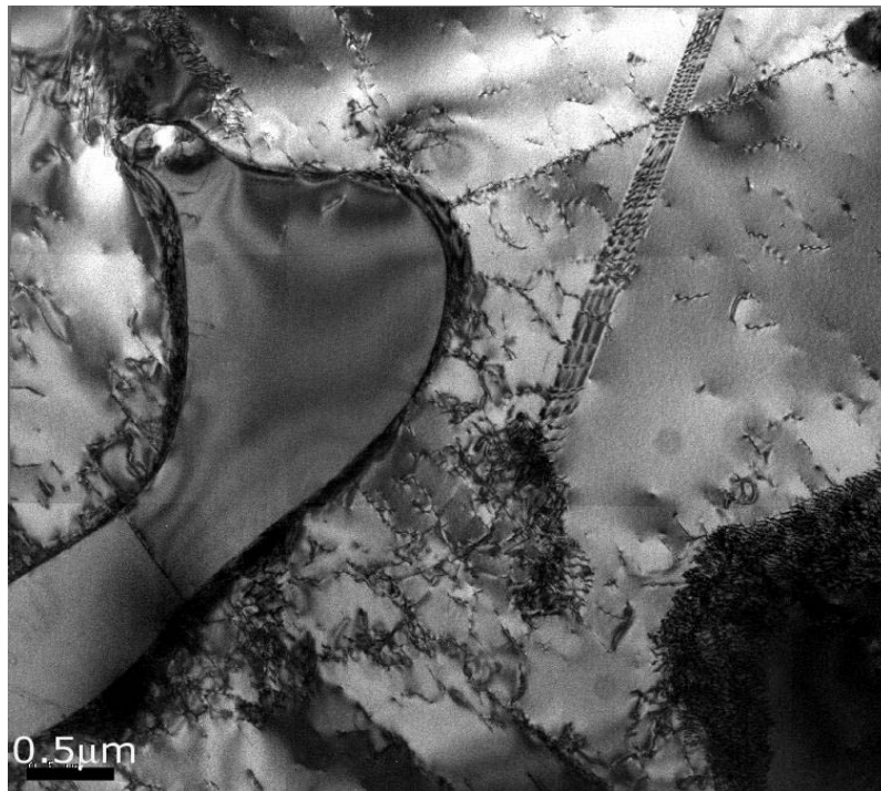
Figure 3.43. AISI 347 heat affected zone.
