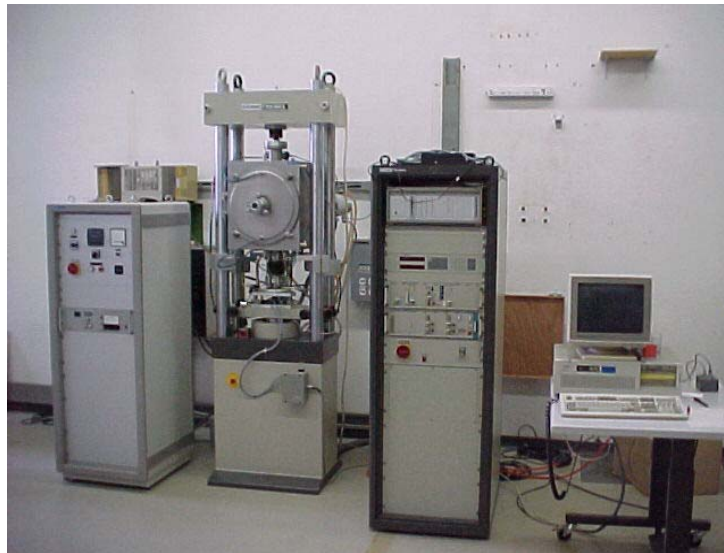
Figure 2.8. The SCHENCK RMC 100 tensile testing machine.
