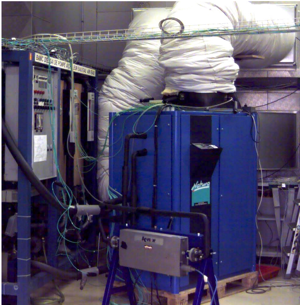
Figure 3: Air-water heat pump test rig at the Laboratory of Industrial Energy Systems at EPFL.
