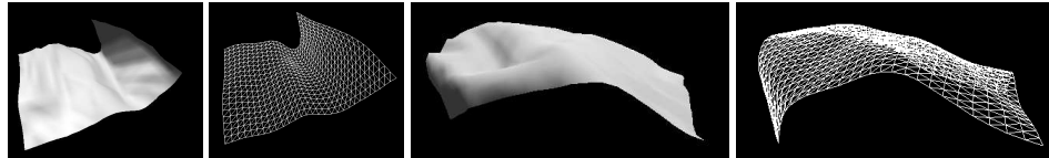
Figure 5: Fitting surfaces created by varying all sets of angles simultaneously. The original shapes are shown as shaded, while the fitted ones are displayed as wireframes.
