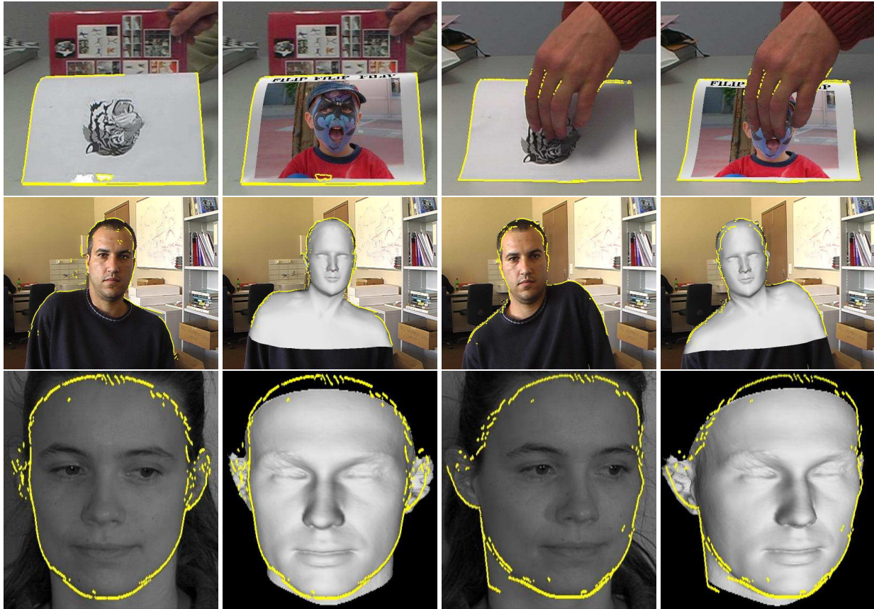
Figure 1: Detecting and using silhouettes for tracking and reconstruction from monocular sequences. The detected silhouette points are shown in yellow, or white if printed in black and white. First row: Tracking a deforming piece of paper with a tiger on it and replacing the tiger by a picture, which involves accurate 3-D shape estimation. This is done in spite of the moving book and the occluding hand. Middle row: Tracking the head and shoulders of a moving person. The reprojected 3-D model is shown as a shaded surface. Note that, even though the background is cluttered, we did not need to perform any kind of background subtraction. Bottom row: Precise reconstruction of a face from a short sequence in which the subject faces the camera.
