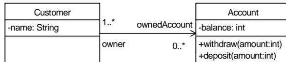
Fig. 2: A UML Class Diagram
