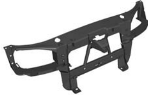
Figure 4-1: Front subframe system of Ford Mondeo
