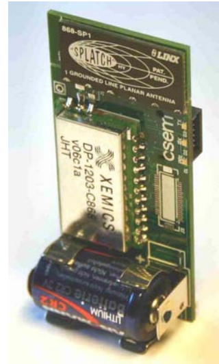
Figure 7.3: WiseNode: A miniaturized low power wireless sensor node based on the XE1203 radio and the XE88LC06A microcontroller.
