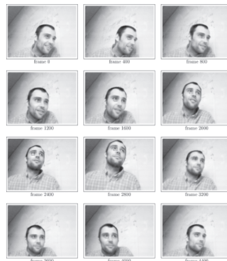
Figure 3. High speed tracking of a gray-level template (32x32 at ~2000 frames per second).
