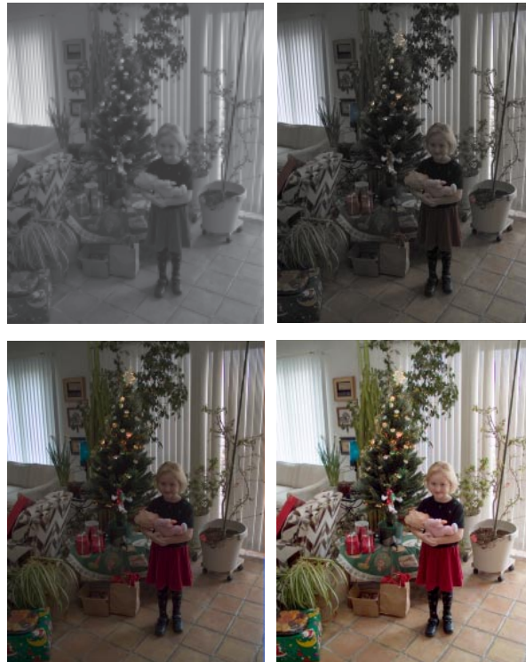
Figure 1. Top left: raw image data with analog dark-current subtraction and gamma = 2.2 encoding nonlinearity, but no analog gains. Top right: "camera RGB" image data, after flare subtraction, white balancing and demosaicing (displayed using gamma = 2.2). Bottom left: scene-referred image data, after matrixing to scRGB color space (displayed using gamma = 2.2). Bottom right: sRGB image data, after color rendering and encoding transforms.
