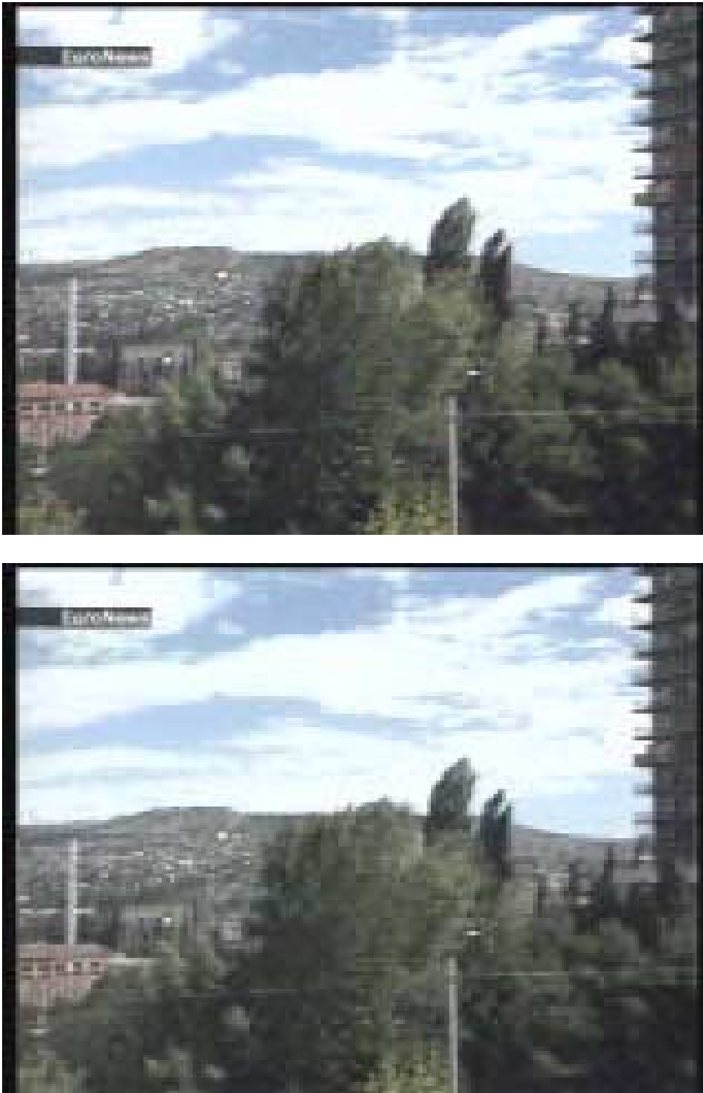
Fig. 12. Sample reconstructions. Top: an original frame from a GOP with a significant amount of motion (the camera is panning over a relatively complex scene, with rich textures); bottom: a frame from the GOP reconstructed by lcavpc35 in 0.6 seconds. The PSNR for this GOP is 33 dB—in real-time playback, it is impossible to tell the difference between the original frame and the reconstructed one.
