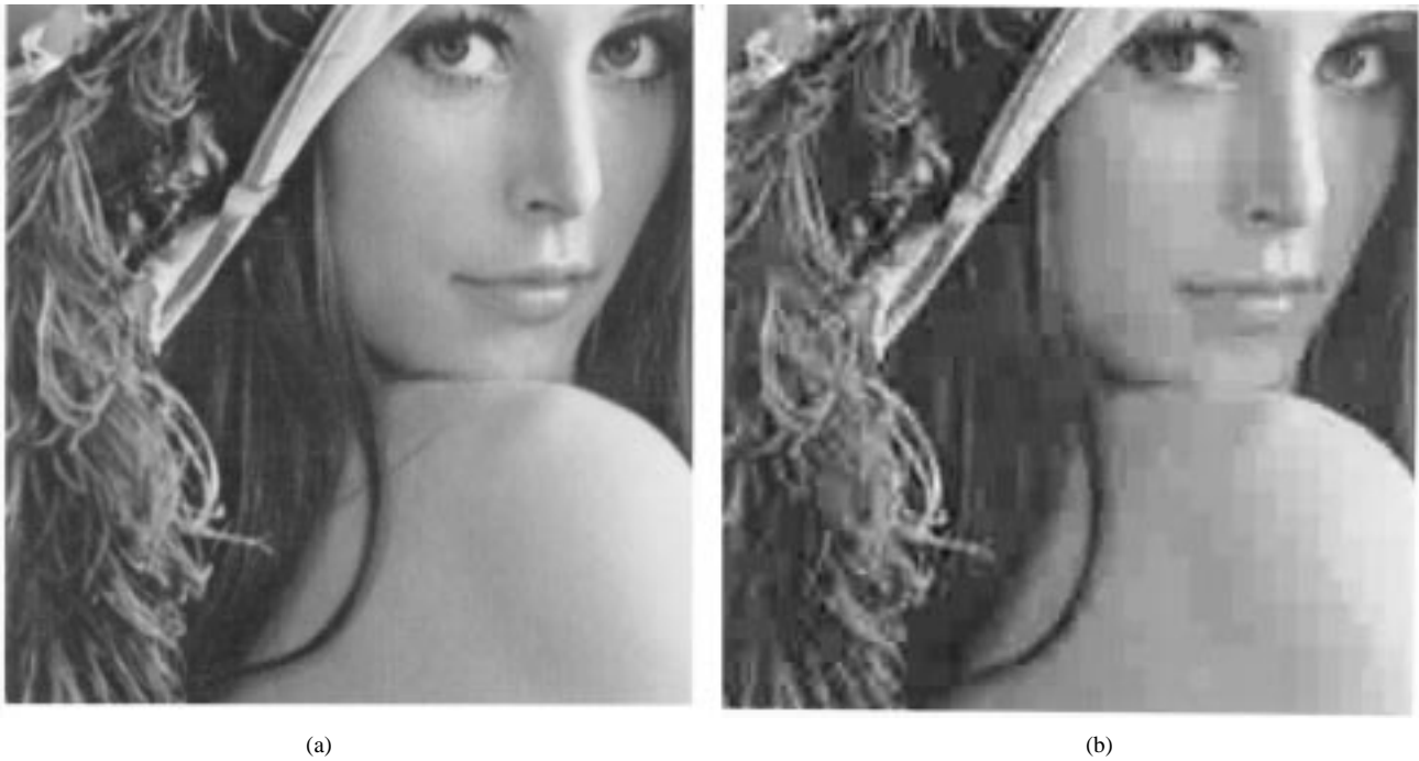
Fig. 4. DCT coding. (a) Original 512 \times 512 image. (b) DCT decoded image at bit rate 0.25/pixel (PSNR = 30.15 dB).
