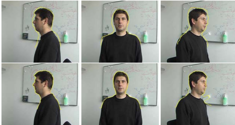
Figure 5.2: Silhouette detection using active contours: Top row: Manually outlined initial guesses used as an input for snakes algorithm. Bottom row: Final silhouette contours after the snake algorithm converged. Note that in the last image snake was attracted by the strong edges of the background.
