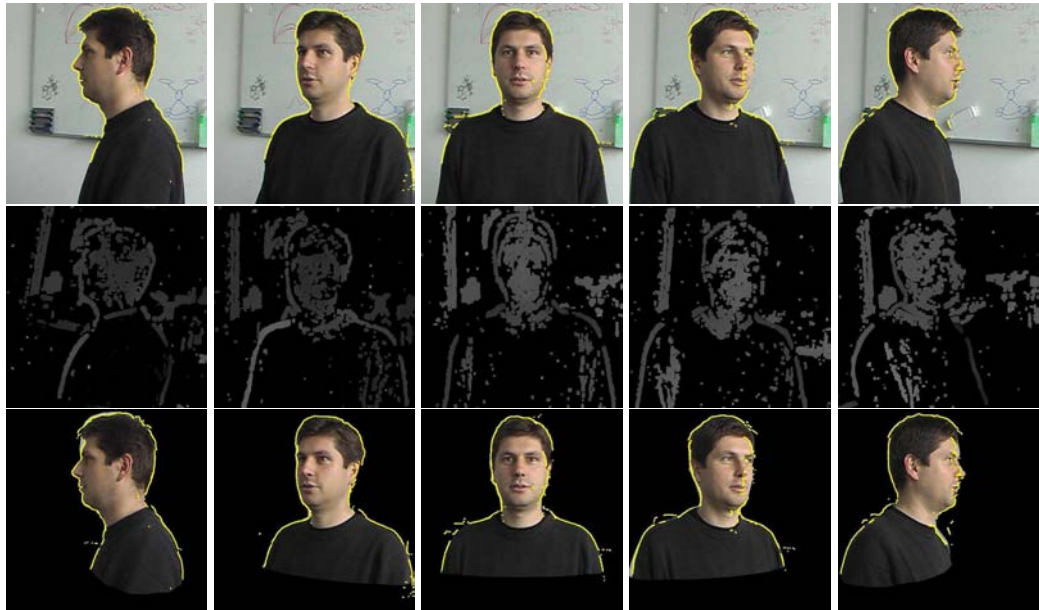
Figure 7.6: Reconstruction from an uncalibrated video sequence. Top row: 5 of 14 images from a short video sequence with overlaid silhouettes for the neck and shoulders. Middle row: Disparity maps computed from the image using a correlation-based stereo algorithm, after automated registration. Bottom row: Textured reconstructed models obtained by using a triangular implicit mesh model for the upper body.
