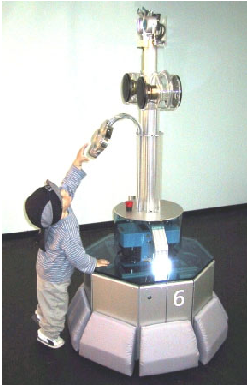
Figure 3.1: Robox was developed at the Autonomous Systems Lab for tour-guiding during the Robotics@EXPO.02 event.
