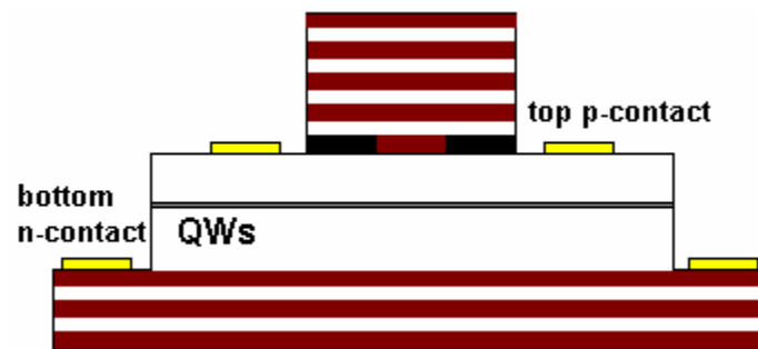
Figure 1.10: Schematic view of an intracavity contacted oxide-apertured VCSEL.
