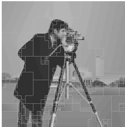
Figure 4.7: Prune-join quadtree tiling for the cameraman image at bitrate=0.071 bpp.
