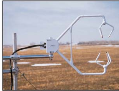
The CSAT3, shown making measurements over a fallow field in Minnesota, provides precision turbulence measurements with minimal flow distortion.
