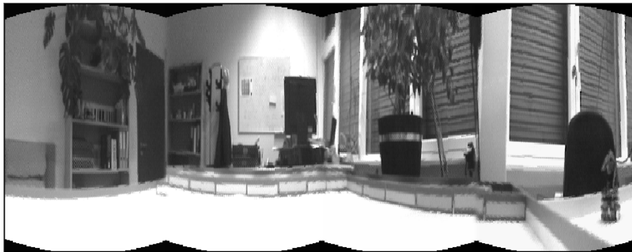
Figure 5.2: A view taken by the Khepera in the “Office” environment. Four camera images are merged into one panoramic view, covering about 240^\circ .
