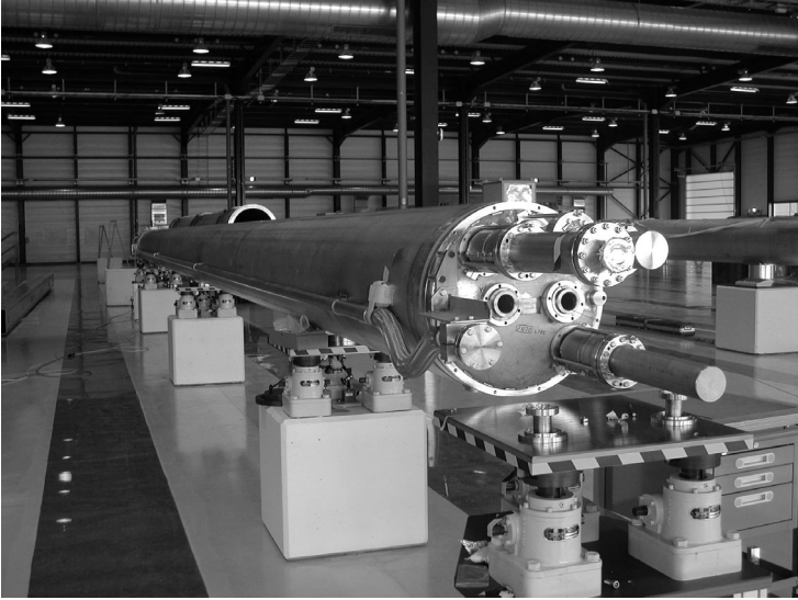
Figure 5-14. One of the 1232 main superconducting dipoles of the future LHC, before the installation of the heat insulating layers. Mass : 23.8 t, length : 15 m.
