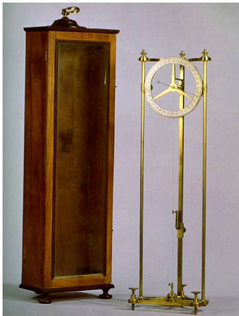
Figure 2.2 Early example of a Saussure hygrometer (by J.J. Miranda, Coimbra).
