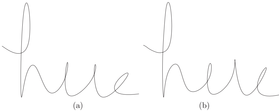
Figure 5.7: Non-uniform to uniform grid conversion. The number of uniform sampling points is 26. (a) Standard method: Peak SNR= 32.934 dB; (b) Projection method: Peak SNR= 34.820 dB. The word is readable here.
