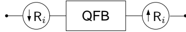
Figure 3.9: Quincunx filter banks with resampling operations that are used in the DFB starting from the third level.
