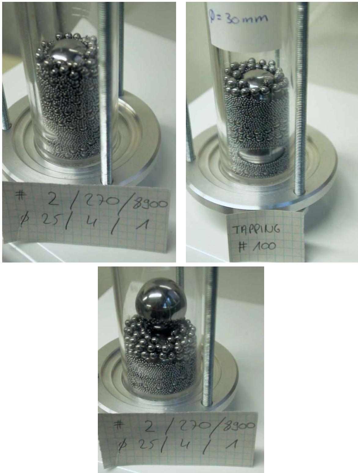
Figure 5.36: Spheres of 1mm, 4mm and 25mm in cylinders of 30mm (top, left and right) and 36mm (bottom).
