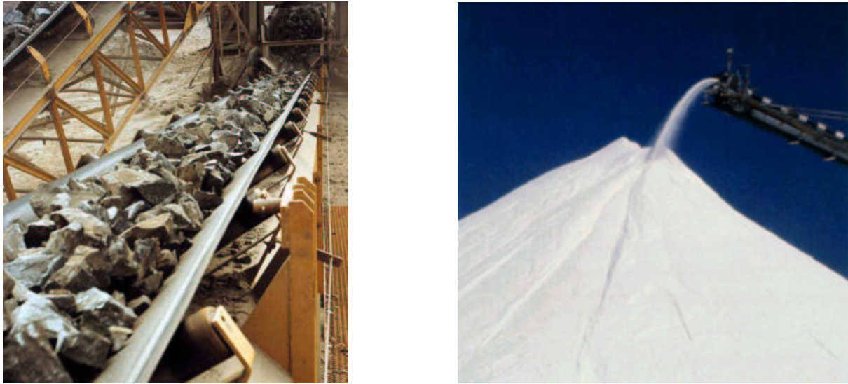
Figure 1.1: Two examples of industrial processes involving granular materials: transportation by conveyor belt and storage.
