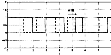
Figure 3.6: Shifted bilevel signal with two transitions in the interval [5, 6].
