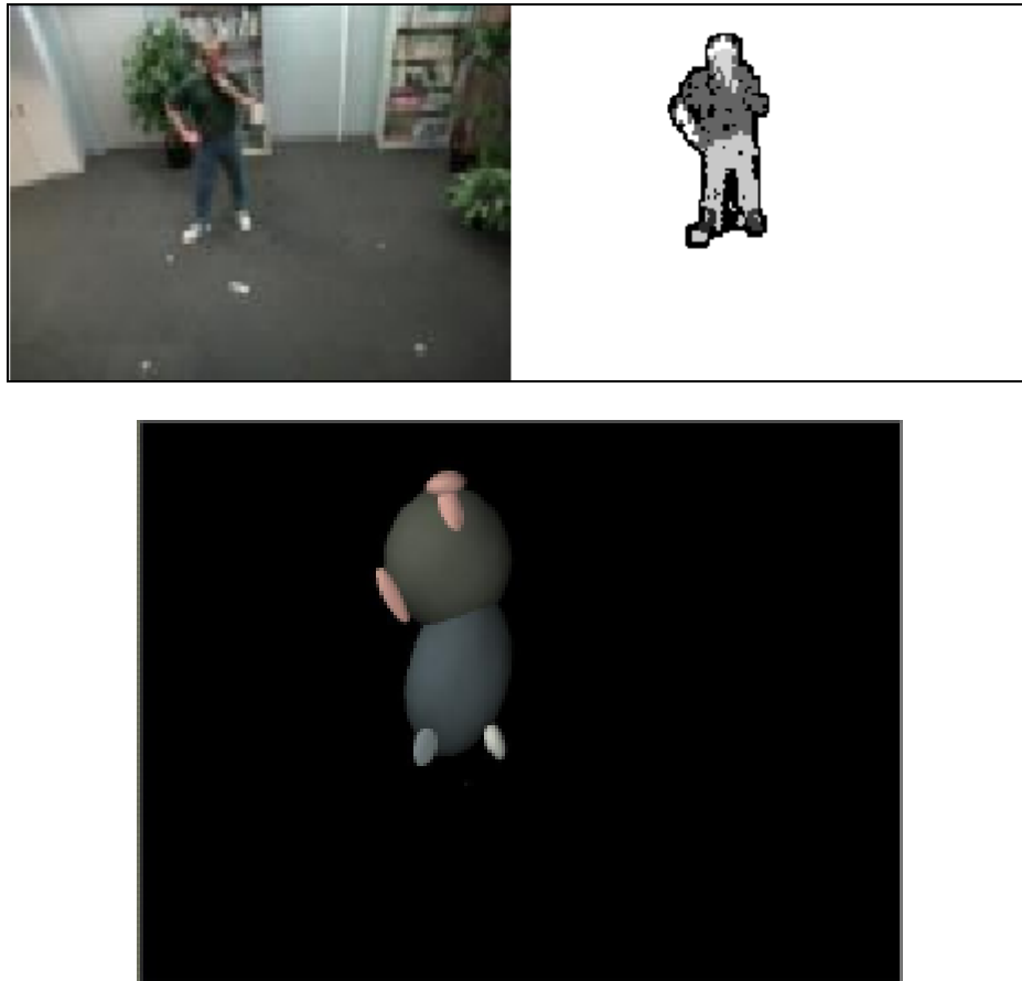
figure 3.11 – Pfinder: human figure extraction and blob-based model
