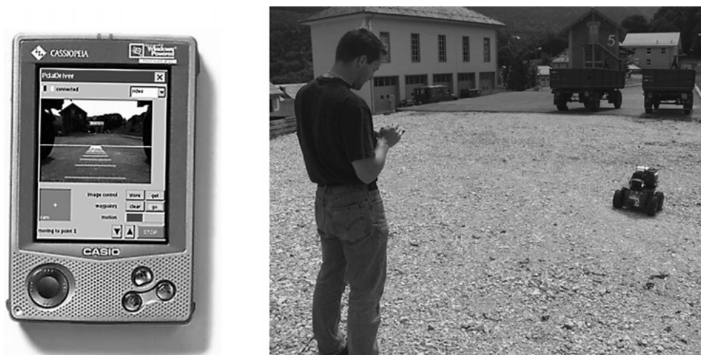
Figure 6. PdaDriver: user interface (left), remote driving a mobile robot (right).
