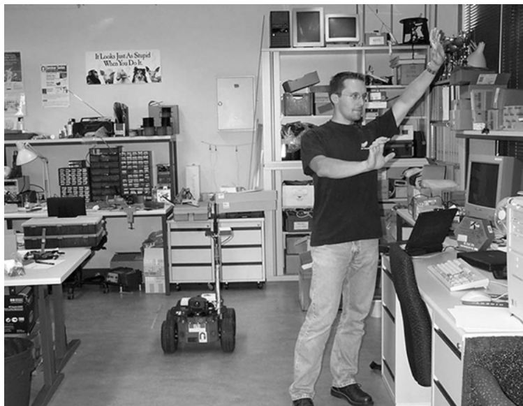
Figure 5. Visual gesturing for vehicle teleoperation.
