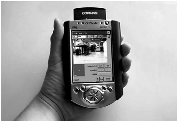
Fig. 3. PdaDriver is a personal digital assistant interface for vehicle teleoperation.
