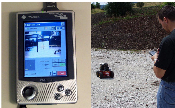
Figure 2. PdaDriver: a personal user interface for collaborative human-robot exploration
