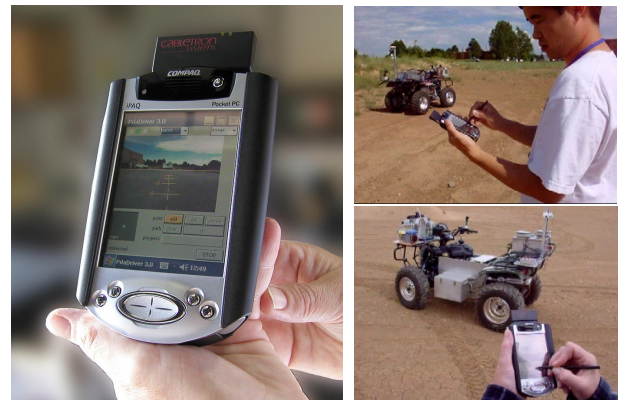
Figure 1: Left , PdaDriver (version 3) on a Compaq iPAQ; right , Remote driving with PdaDriver
