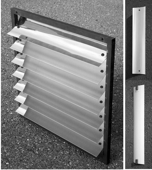
Figure 1: Venetian blind prototype presenting curved slats with mirror and diffuse beige coatings on their upper and lower faces respectively.
