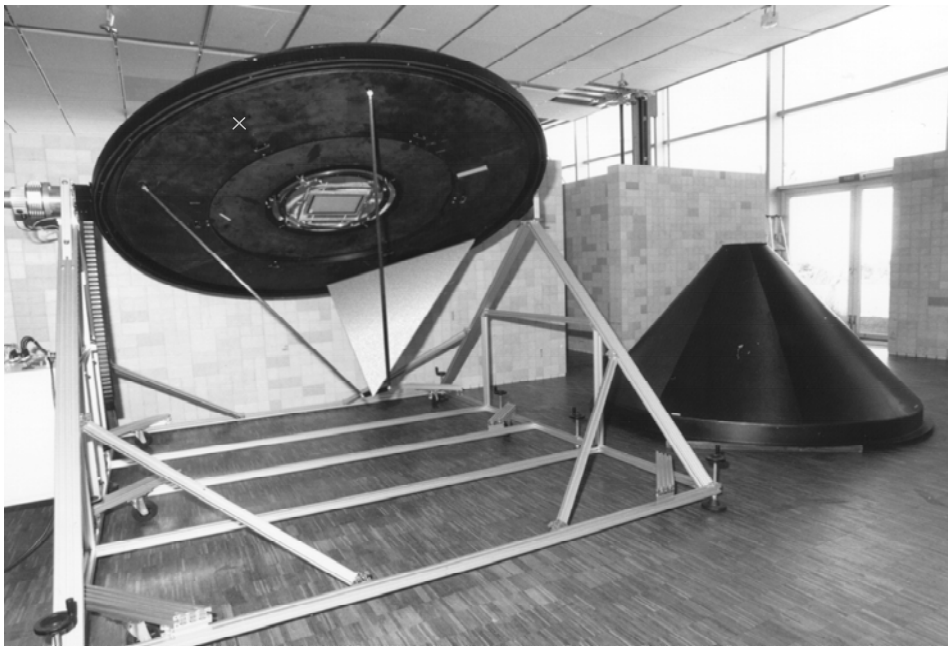
Fig. 3.1. View of the bi-directional photogoniometer. The light detection device is mounted behind the adjustable moving plate and protected against parasitic light by a lightproof cache (placed on the floor for convenience). The CCD camera (absent in this picture) is fixed on the rotating ring at the cross mark.
