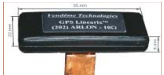
This GPS antenna for pedestrian navigation is a miniaturized plate antenna with controlled impedance. Its characteristics allow remaining in the frequency workspace even when the center frequency varies because of the presence of the human body. For testing purposes, the antenna was adapted and coupled with a modified 20dB enhancer.
