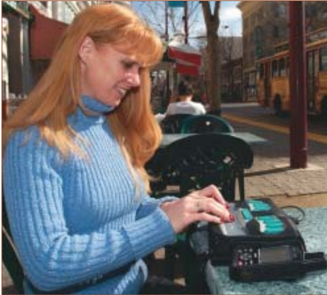
The PNM directly outputs NMEA messages that will be read by the BrailleNote GPS module. BrailleNote GPS is a fully accessible Braille or talking GPS for people who are blind or visually impaired.
