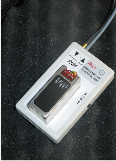
Figure 9: The latest prototype also integrates a gyroscope, necessary for indoor navigation as well as navigating in magnetically disturbed areas.
