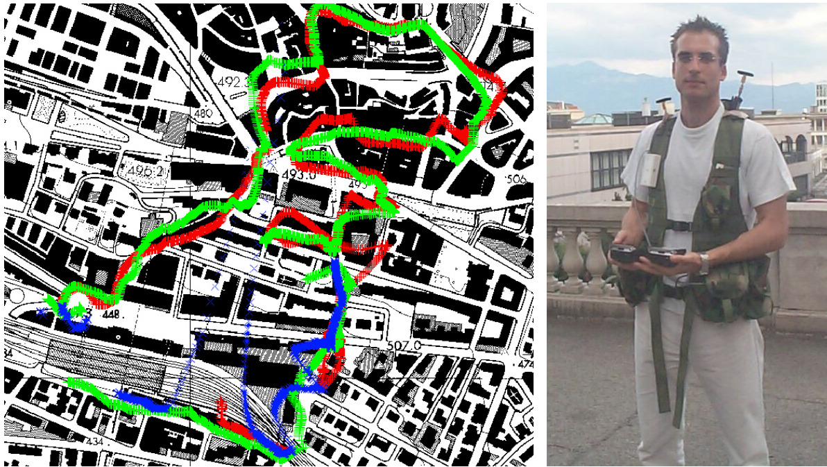
Figure 16: : Left : Trajectory downtown Lausanne with simultaneously 3 GPS receivers from u-blox AG, Switzerland, using 3 different antennas. In blue, a commercial patch antenna, in red a special helicoidal antenna made by Sarantel Ltd (UK) and in green a specific linear antenna developed by Vendôme Technologies (France). Right: The author during the tests, wearing two PNMs (in the front and in the back) as well as two single GPS receivers.
