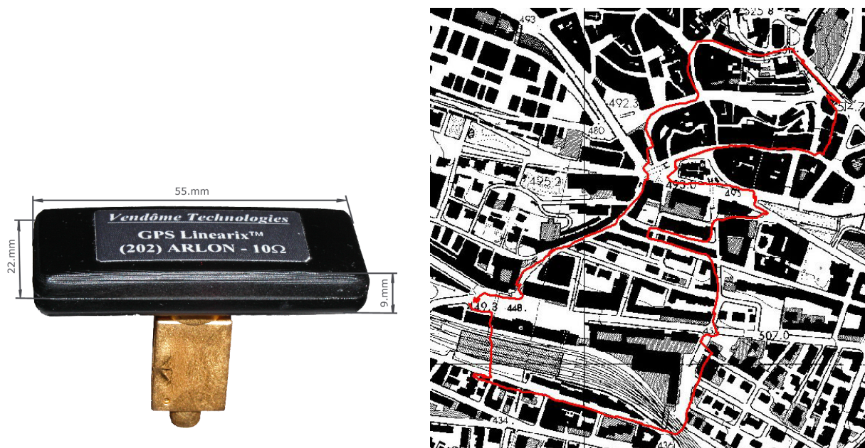
Figure 17: Left: This specific GPS antenna for pedestrian navigation has been developed by Vendôme Technologies (France). It is a miniaturized plate antenna with controlled impedance. Its characteristics allow remaining in the frequency workspace, even when the central frequency is shifted because of the presence of the human body or other disturbing objects. For the testing purposes, the antenna has been adapted and coupled with a modified 20dB amplifier from Sarantel Ltd (UK). Right: Continuous and unique representation of the Figure 13 trajectory output by the PNM. Only 5 GPS positions were used during the whole run to calibrate the different models and bound the statistical error.
