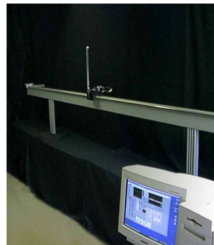
Figure 1. a) The electrical drive consists of DC motor equipped with a built-in tachometer and a potentiometer connected to the motor axle for measuring the angular position. b) The 4 meters long inverted pendulum is equipped with two absolute digital encoders, the first one measuring the cart position and the second one the arm angle.
