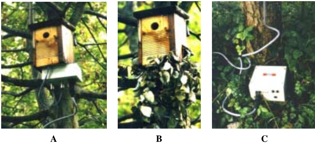
Figure 2. A NMAS installed in the field. (A) Nest box with embedded sensor module (modified door) and sensor processing and data logging module (placed beneath the nest box). (B) Camouflaged with leafy branches. (C) Power unit and user interface at the foot of the tree.
