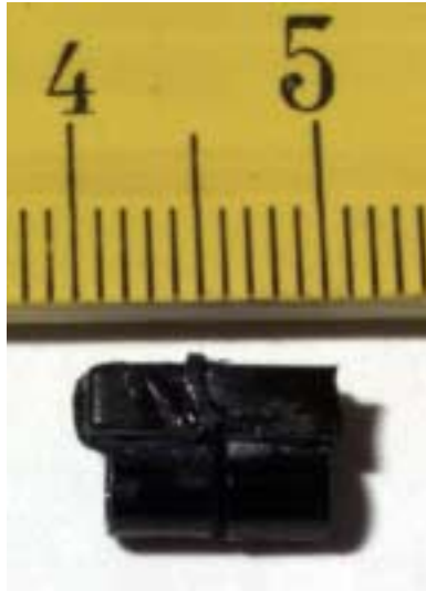
Figure 3. The PIT tag attached to the bird's leg. It consists of a passive transponder and two plastic rings. The three pieces are bound together with cotton wire and glued (scale 1 cm).
