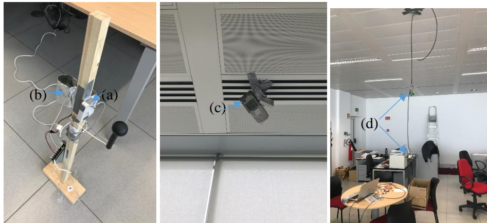
Picture 4 - (a) – HOBOT data logger sensor on wooden pole; (b) – K-33 sensor on wooden pole; (c) – Hobo with screen near the inlet; (d) – CO 2 measurements stratification cable
