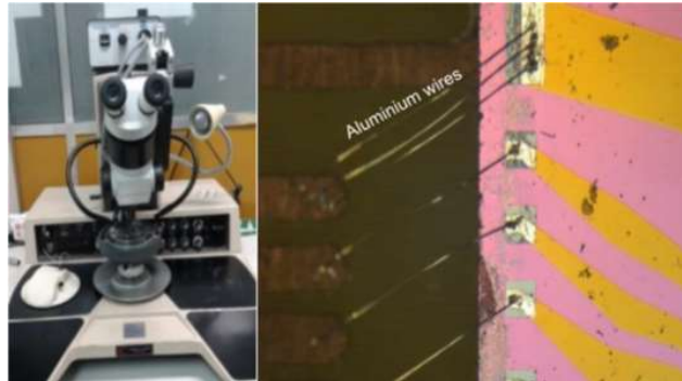
Figure 3.17 - Wirebonding system and connection of aluminum wires between PCB and chip.
