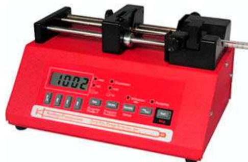
Figure 7.3 - New Era NE-1000 Series programmable syringe pump used for the flow regulation.
