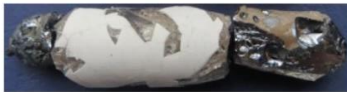
Figure 2.7 - A small mc-Si ingot grown in a fused silica crucible without coating. The wetting by molten silicon caused considerable sticking [32].
