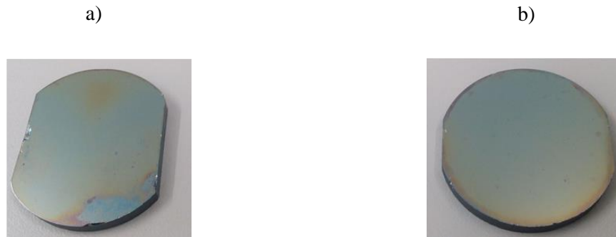
Figure 4.3 - Silicon test samples annealed in Nabertherm LHT 04/18 up to 1200 °C, during 60 minutes with an argon flow of a) 250 L/h (20 °C, 300 mbar) b) 500 L/h (20°C, 300 mbar).
