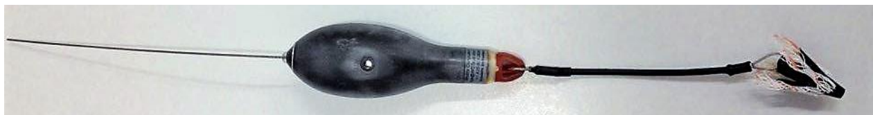
Figure 1.6 - Pop-up Satellite Archival Tag (PSAT) built by Wildlife Computers.
