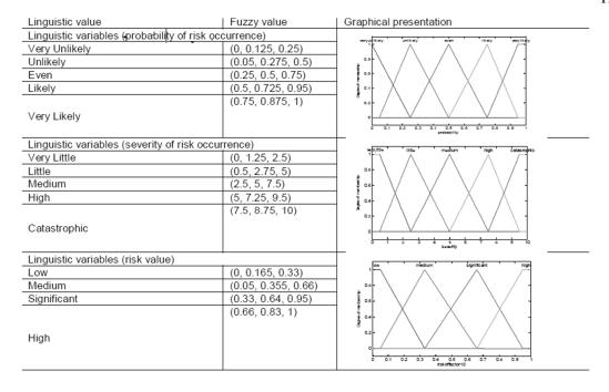
Figure A1. Linguistic and fuzzy values. From Risk assessment of construction projects using network based adaptive fuzzy system, by M. Ebrat and R. Ghodsi, 2011, p. 413. Retreived from International Journal of Academic Research. Reprinted with permission.
