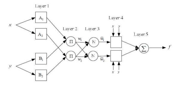
Figure 23. Neuro-fuzzy adaptive assessment model. From *Risk assessment of construction projects using network based adaptive fuzzy system*, by M. Ebrat and R. Ghodsi, 2011, p. 414. Retreived from International Journal of Academic Research. Reprinted with permission.
