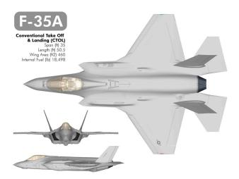
Figure 1. F-35A conventional takeoff & landing (CTOL). From "F-35 Variants," by F-35 Lightning II Program, n.d., retrieved from http://www.jsf.mil/f35/f35 variants.htm
