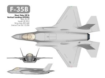
*Figure 2.* F-35B short takeoff & vertical landing (STOVL). From "F-35 Variants," by F-35 Lightning II Program, n.d., retrieved from http://www.jsf.mil/f35/f35\_variants.htm
