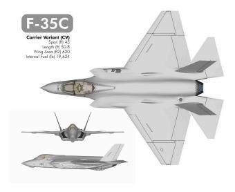
Figure 3. F-35C carrier variant (CV). From "F-35 Variants," by F-35 Lightning II Program, n.d., retrieved from http://www.jsf.mil/f35/f35\_variants.htm
