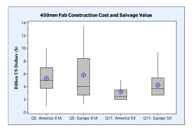
Figure 14. 450mm wafer fab construction cost and salvage value.
