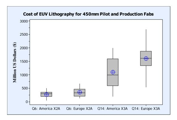
Figure 17. Cost of EUV lithography for 450mm pilot and production fabs.
