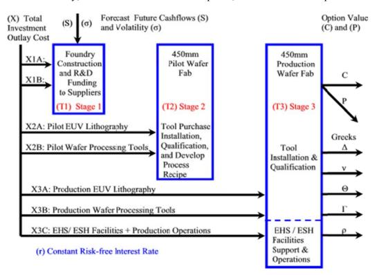
Figure 5. A three-stage compound real option for the 450mm wafer foundry.
