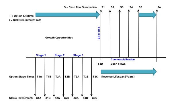
Figure 1. Real option cash flow diagram to determine net present value (NPV).
