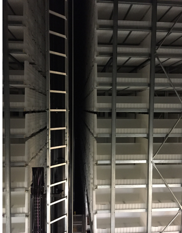
Above left: An SRM waiting for its next job, surrounded by the roller conveyors that feed it. Above right: The upper section of the same crane; the ladder is for maintenance. The foremost containers remain empty. Below left: A barcoded container stocked with unbarcoded print serials. Below right upper: The workstations (one clearly visible bottom-right) outside the voids. Below right lower: Roll cages not dissimilar to those used by supermarkets are transported by the daily Boston Spa-St Pancras shuttle vehicle.
