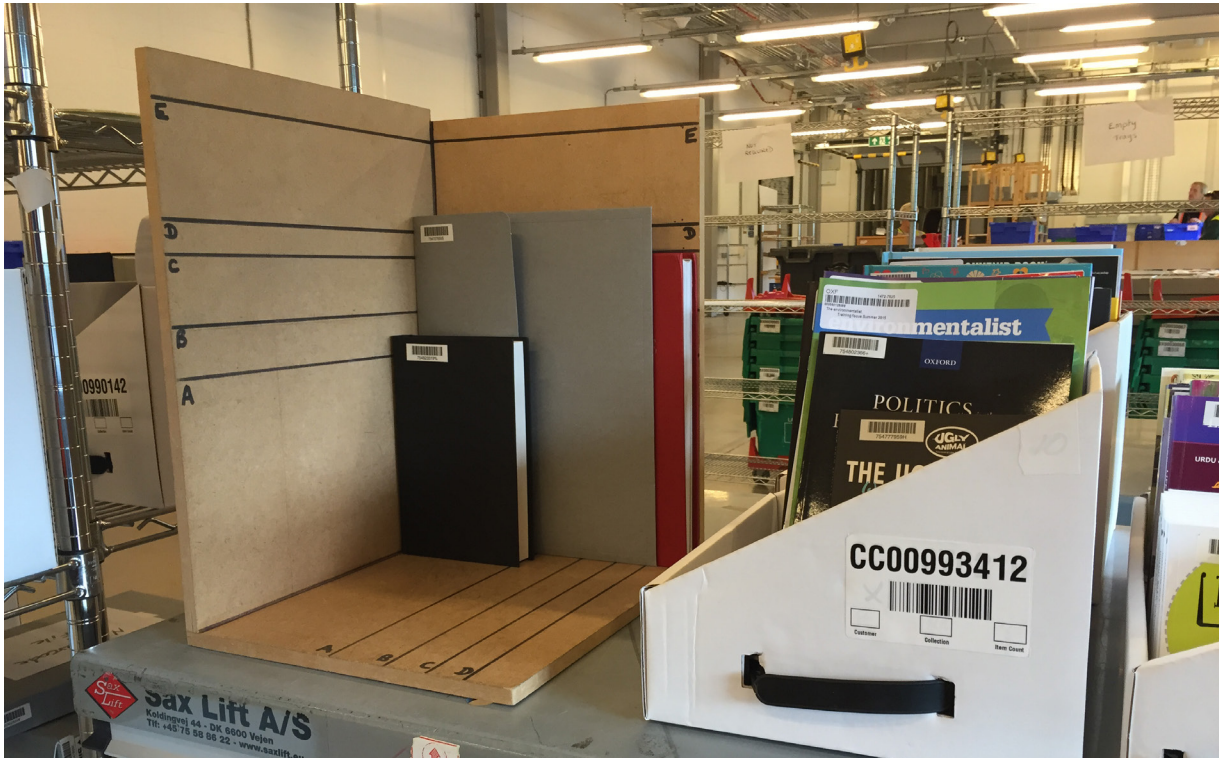
Above: The Nicholson Classification sorter (left) and examples of loaded trays (right). Barcodes are clearly visible on items and trays. Below left: A well-stocked aisle. Below right: From this angle the loaded racking appears to be almost like a conventional bookcase.
