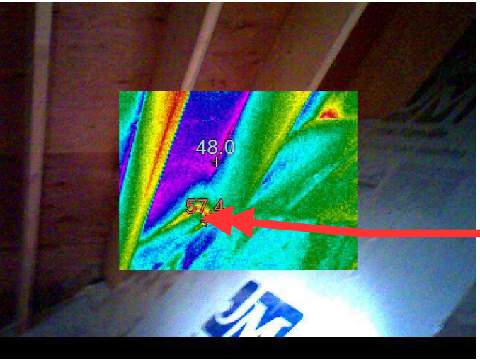
Looking west in the attic toward the northern valley which overlays the exhibit room. Yellow and reds show air-leaks associated with the framing intersection between the exhibit room ceiling/roof and the connector roof.
