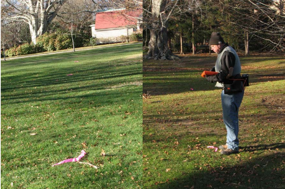
Figure 5: Markers indicate one of the lines laid out for gathering VHF data. The geologist walks the line with the ABEM WADI instrument which gathers data relative to the behavior of the radio waves at water- and non water-bearing underground structures.
