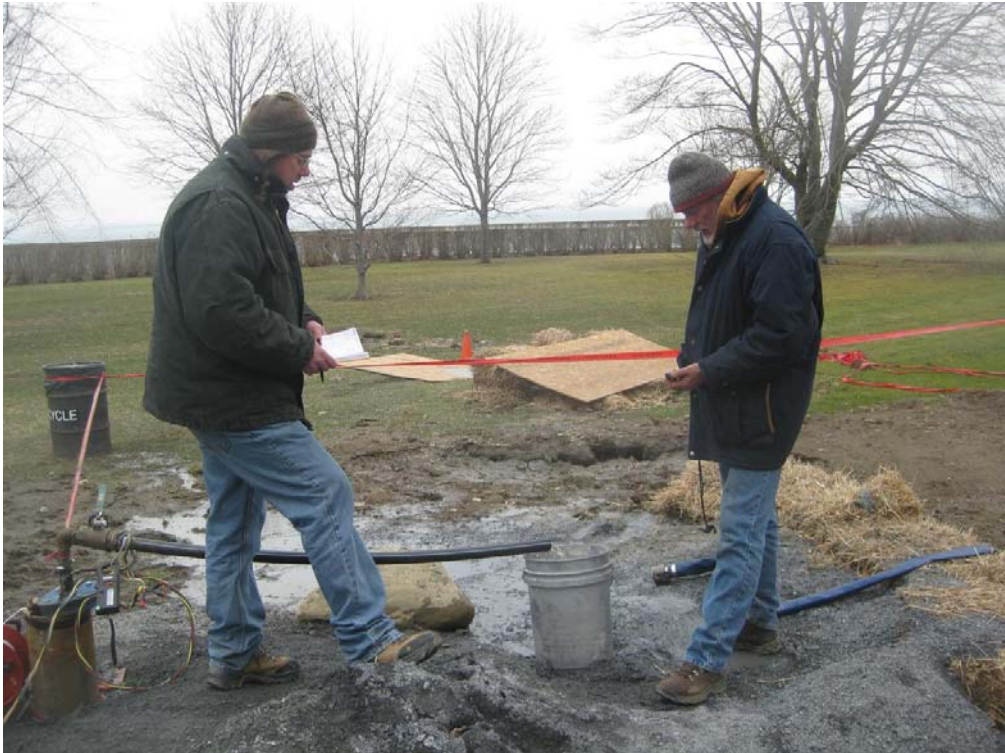
Figure 17: Chris Covell and Joel Russell perform initial rating of gallons per minute.
