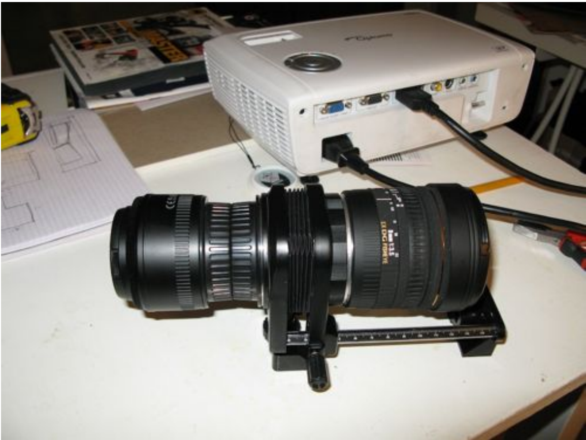
Domebase fisheye lens assembly – 50mm lens on the left, 8mm fisheye on the right
