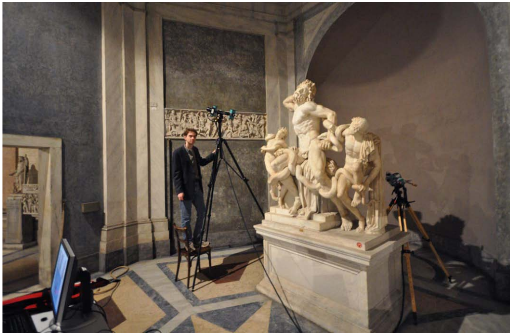
Figure 1: 3D scanning the Laocoön statue group
