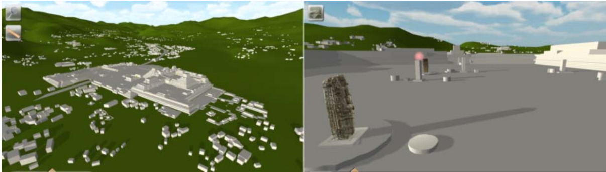
Figure 24. Navigation modes for the QueryArch3D tool: [left] aerial view displaying LoD1 models only, [right] walkthrough mode, with mixed LoD1-to-LoD3 models. An example of the detail view for LoD4 models is given in the next figure (bottom-right).
