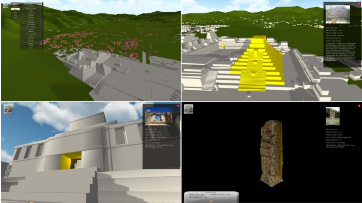
Figure 25. Different data interrogation modes in QueryArch3D. [Top-left] Query by attributes and display of the results in terms of geometries. [Top-right and bottom] LoD-dependent queries on geometric models: at LoD1, only global attributes are shown, for LoD2 to LoD4 models also subparts can be selected and more detailed information is retrieved.
