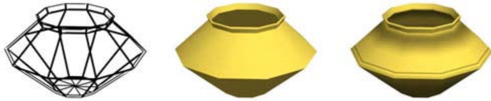
Figure 1: From left to right, a model of a pot without a texture map, with a standard texture map, and with baked texture map.
