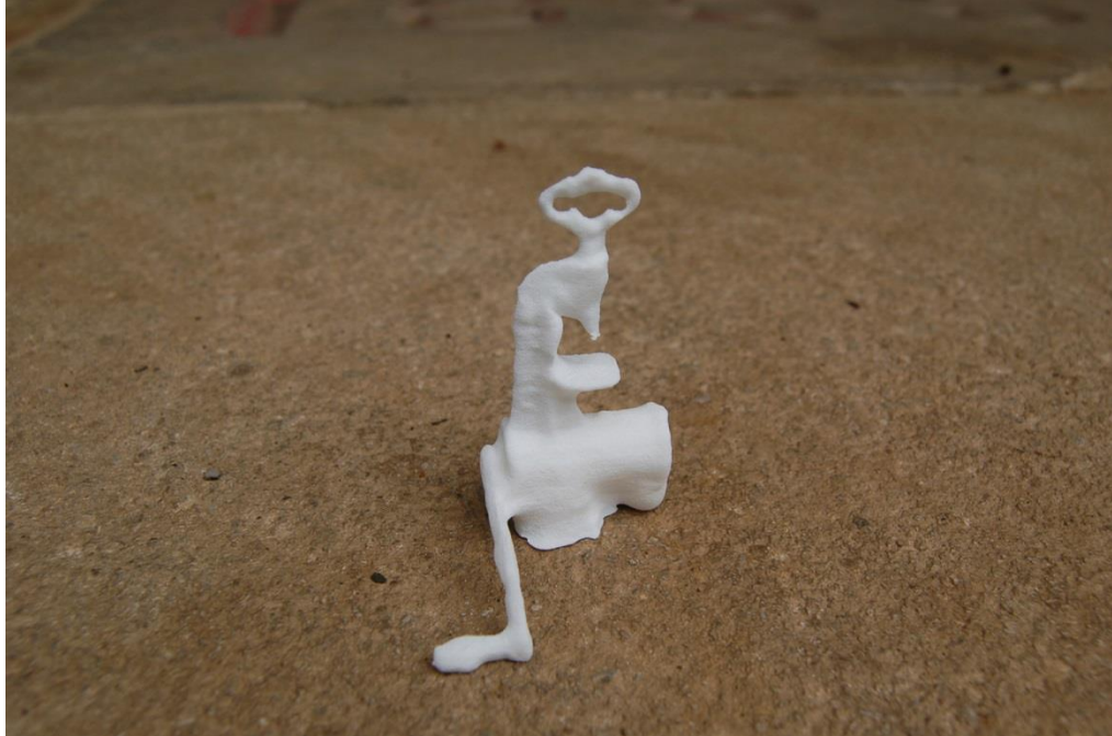
Photograph 15. Printed meat grinder, angle similar to the photoset used for model generation. The photographs of the printed model were all taken outside on my front porch using the Nikon DSLR.
