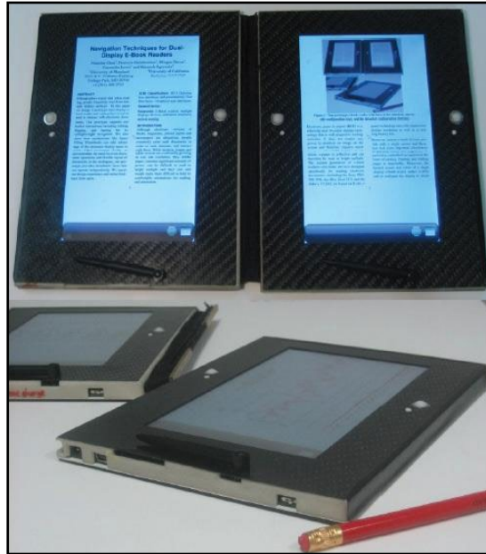
The dual display reader with screens attached side-by-side (top) and detached (bottom) Photo credit: Chen et al. 2008
