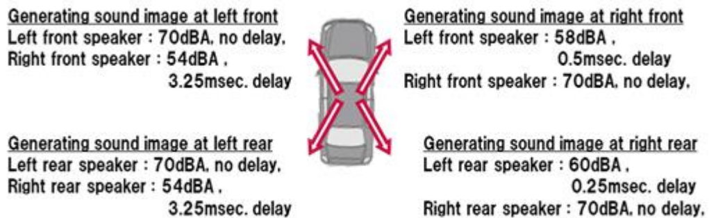
Fig.4-14 Sound Pressure Level and Delay setting for making sound image in driving simulator cockpit
